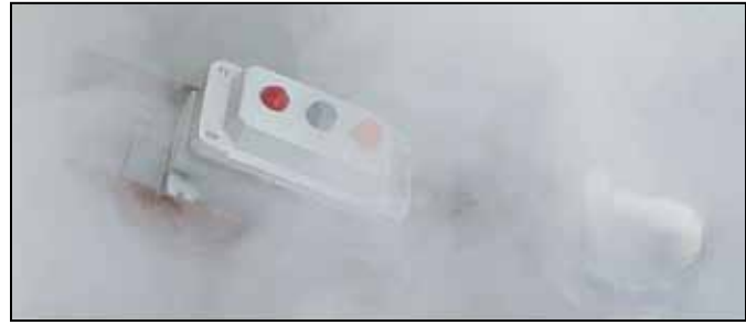
SALINE MIST CORROSION TEST IN OUR LABORATORIES.
